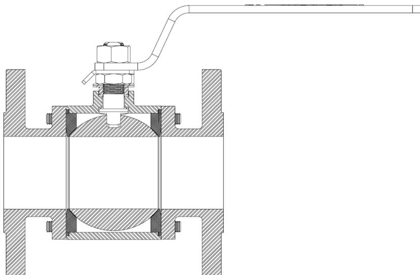
Figura1 – Corte transversal VET Flange Classe 150.
